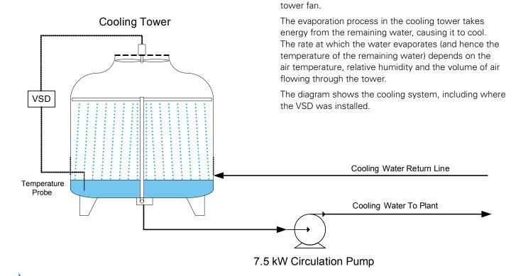
The heated cooling water enters the cooling tower
