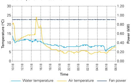
Cooling water temperature, ambient air temperature and fan power. Fan not on VSD
